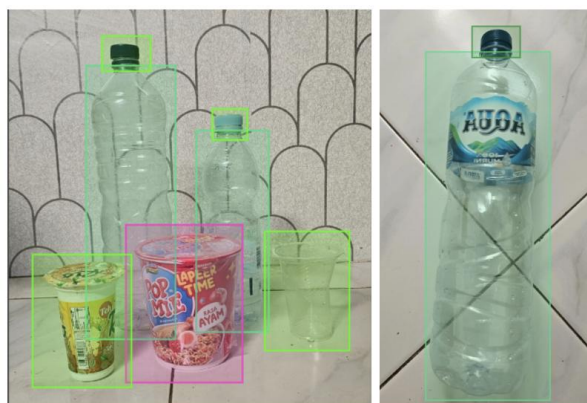
Figure 2. YOLO-annotated plastic waste components with individual bounding boxes.
